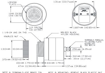
NOTE A: TERMINALS-.032 BRASS TIN PLATED, TAPPED FOR #6-32 SCREW. TUD #6-32 NICKEL PLATED BRASS SCREWS INCLUDED. WILL ACCEPT 1/4\* QUICK CONNECT.
